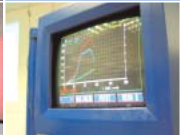
Tyres and rolling road share the punishment, while the workshop fills with the smoke from a roasted and purged exhaust Power and torque production plotted against engine rpm are displayed on a monitor and also projected on to the wall
